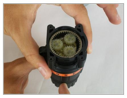
• Twist the gear and see if the three gears rotate without jamming.
