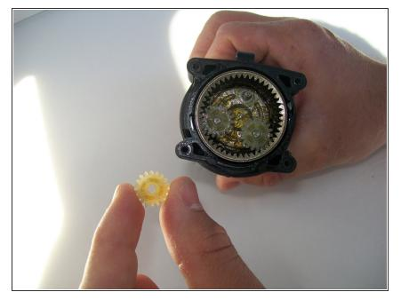
The gear has been removed and now can be replaced by another gear.
