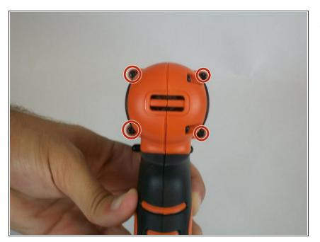
• Remove the four screws on the back top side of the drill.
