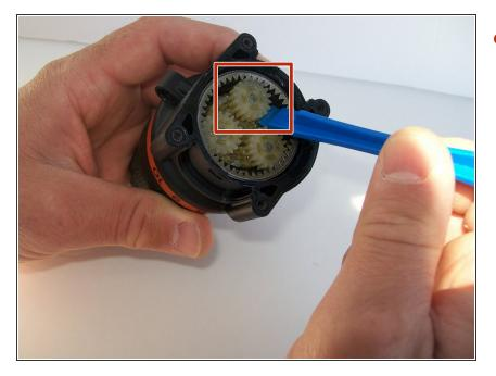
• Using the spudger place it under the gear as illustrated.
