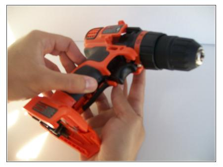
Gently grab both sides of the drill casing, and separate both sides from each other.
