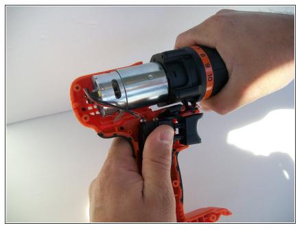
• Gently remove the top part (motor and chuck) from the rest of the drill.
