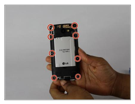
Remove the eight 4mm screws along the side of the mid panel using the Phillips #000 screwdriver head.
