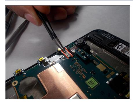
• Locate the camera and its connector.
