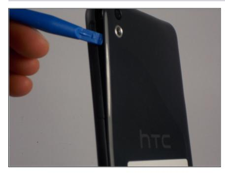
Pry open the back panel by inserting the plastic opening tool on the left of the camera.
