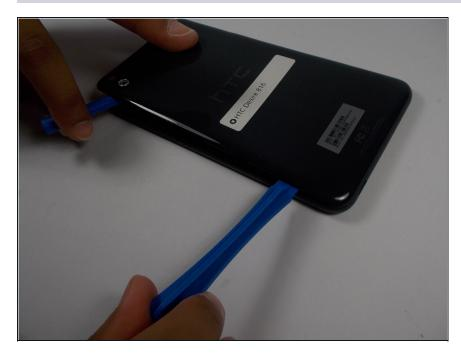
Once you get an open spot, with a second plastic opening tool, slide down to the bottom of the phone to free the rest of side.
