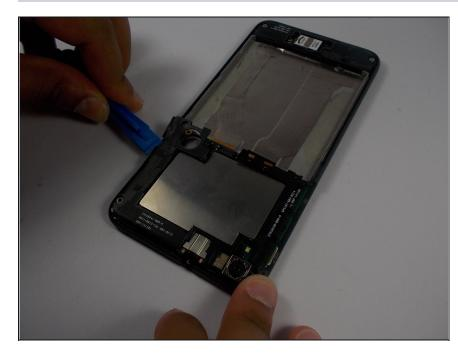
• Remove the black plastic casing with a plastic opening tool.
