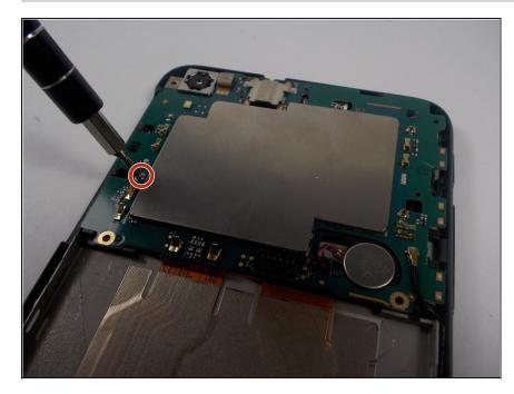
• Using the PH000 screw driver head, unscrew the one screw that is holding down the mother board. (This screw is located on the left side of the motherboard.)
