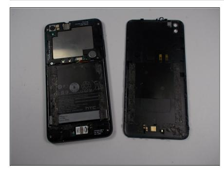
Once all way around the bottom, the panel should be broken free of the adhesive, and the rest of the panel should pop right off.
