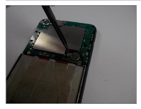
• Using a pair of <u>tweezers</u>, gently disconnect the battery wire from the motherboard.
