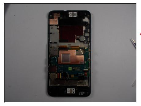
• Lift the motherboard and peel it back.
