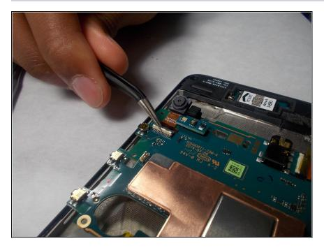
• Using a pair of tweezers, lift the white part of the connector and disconnect the camera from the motherboard.
