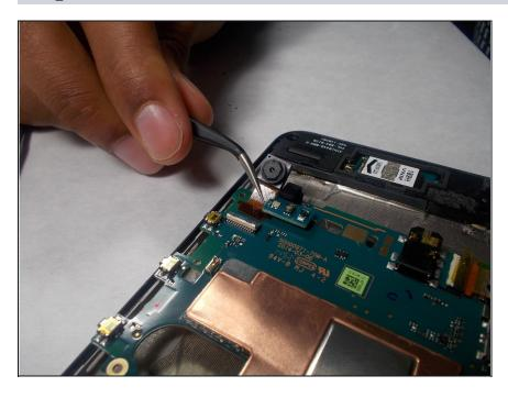
• Use a pair of tweezers to slide the camera out and remove the camera from the device.
