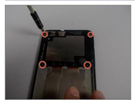
Using the T5 screwdriver, unscrew these four screws in order to remove the plastic casing.
