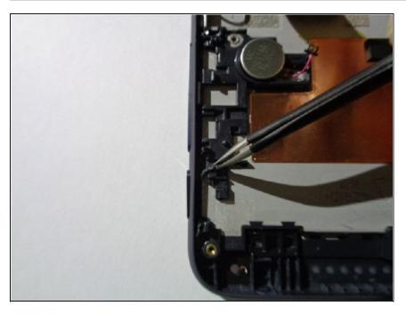
With a pair of tweezers, located the rubber power button piece and pull towards yourself in order to set it free.
