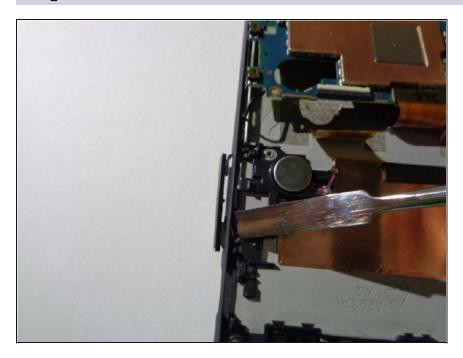
Using a metal spudger, gently push the volume button out.
