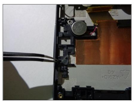
Using the a pair of tweezers, locate the rubber button piece and gently lift up in order to set it free.
