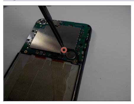
With a pair of <u>tweezers</u> disconnect the battery wire from board.
