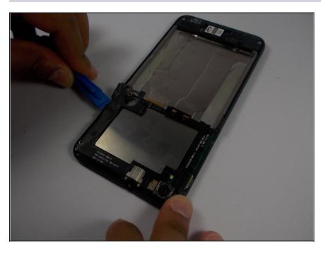
• Lift and remove black plastic casing from the device with a plastic opening tool.
