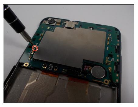
Using the PH000 screw driver, unscrew the remaining screw that is holding down the motherboard. It is located on the left side of the motherboard.
