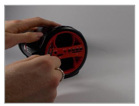
If the screws are difficult to remove, use a pair of tweezers to twist and pick them out.
