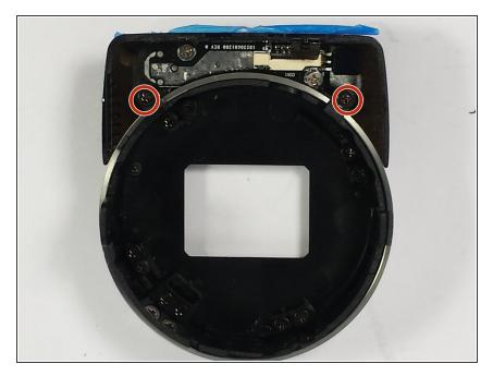
Take out the two 20 mm Phillips #0 screws that attach it to the shutter.
