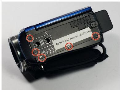
Remove the five 30mm Phillips #0 screws on the bottom of the camera.
