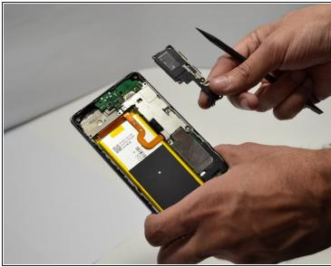
• **Gently**, use the flat end of the <u>Spudger tool</u>, or a metal opening tool to **lift** and **remove** the loudspeaker from the phone. The loudspeaker is the entire portion of the phone where the screws were extracted.
