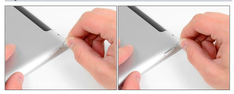
Use a SIM eject tool or an uncoiled paperclip to eject the SIM card tray.
