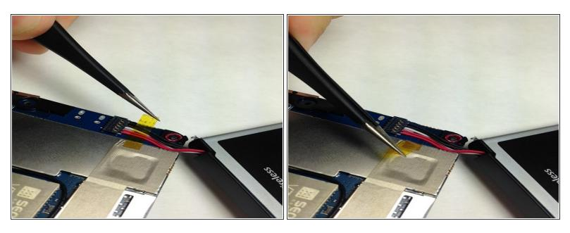
With a pair of <u>Tweezers</u> remove the yellow tape covering the battery wires.
