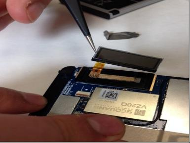
Gently insert the <u>Tweezers</u> underneath the LCD screen and lift the LCD screen off of the circuit board. To reassemble your device, follow these instructions in reverse order.
