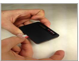
Remove the SIM card, that is located on top of the Jetpack.
