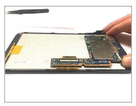
Grip the motherboard and lift up gently and remove the motherboard from the device.
