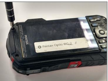
• Remove all four 1 mm JIS #00 screws from the back of the camera.
