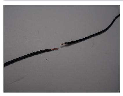
Again, use the wire strippers to strip back a small amount of the rubber coating on the wire.
