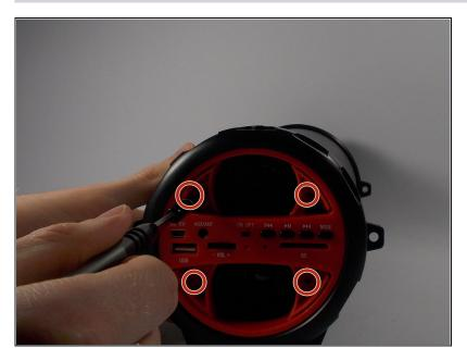
Use a PH1 size Phillips head screwdriver to remove the four 0.7 cm screws.
