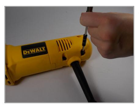
Remove the four 19mm T20 Torx screws at the rear of the device.
