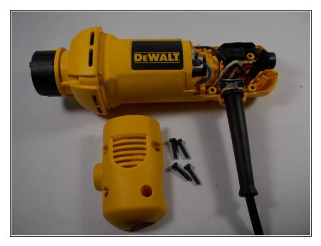
Remove the cover to expose the inside of the tool.
