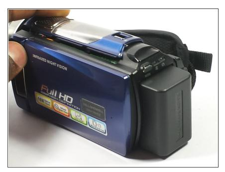
The battery is located on the back of the camera.
