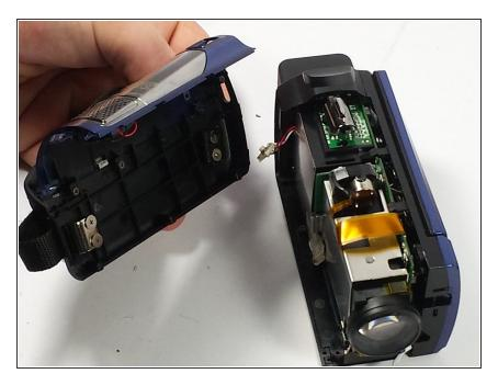
Pull the side with the hand strap upwards to disconnect it from the camcorder.
