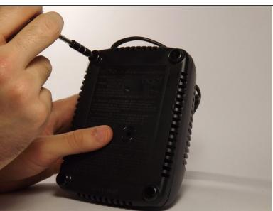
Remove the four 13 mm, Torx Security #15 screws found on the bottom of the charger.
