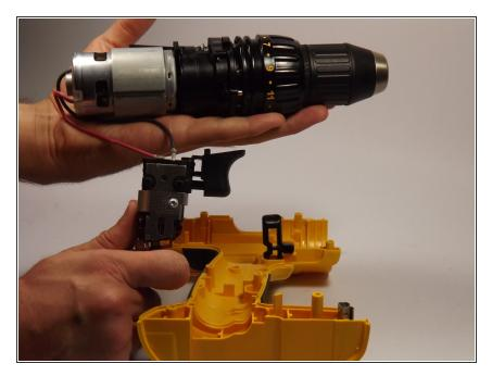
Remove the drill mechanism from the shell.
