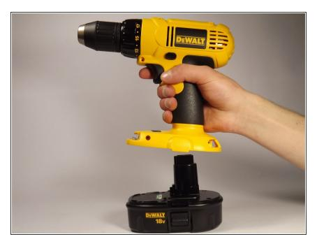
Remove battery from drill.
