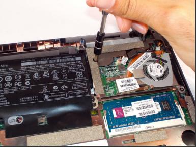
Remove the three 4.0 mm screws with the keyboard indicator next to them using a Phillips #1 screw driver.
