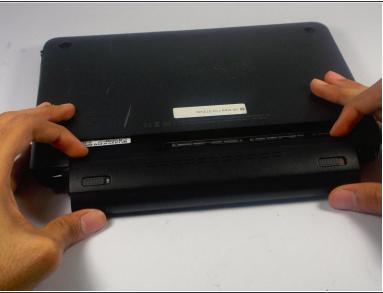
• With the left switch still pushed inward, pull the battery towards you to remove it from the computer.
