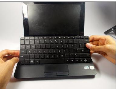
Move and hold the bezel slightly towards the screen while lifting the keyboard from the top.
