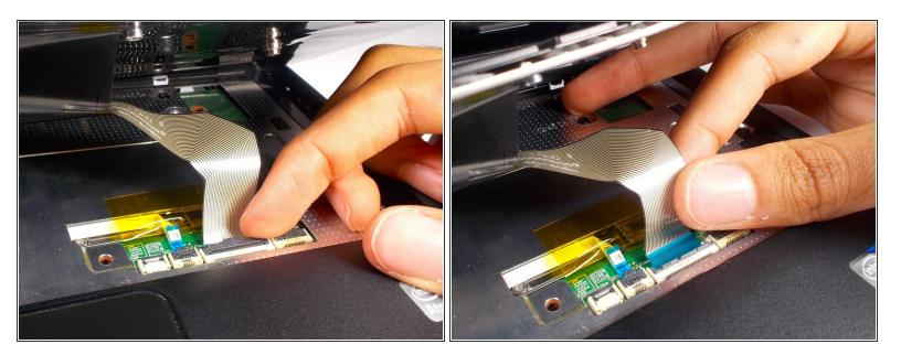
Lift the black holder connected to the keyboard cable until it points up.
