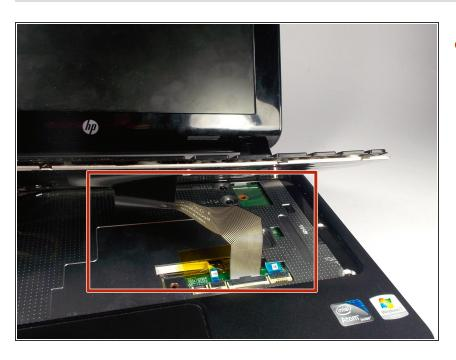
Pull up the keyboard from the bottom corners exposing the keyboard cable.
