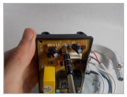
In order to remove the small housing that covers the motherboard, remove the lone screw with a PH1 bit.
