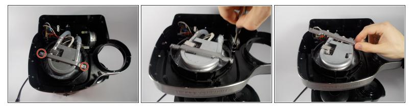
Remove the two .374 inch long Philips head screws from the brace using a PH1 bit and take the brace off.
