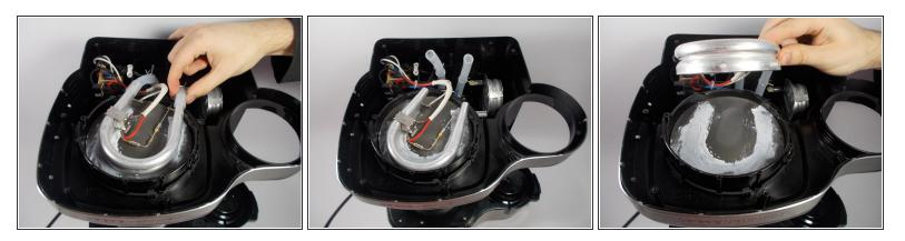
• With the spring clamps moved down, slide the tubes from the ends of the large heating component. Once the ends are free, separate the component from the hot plate.
