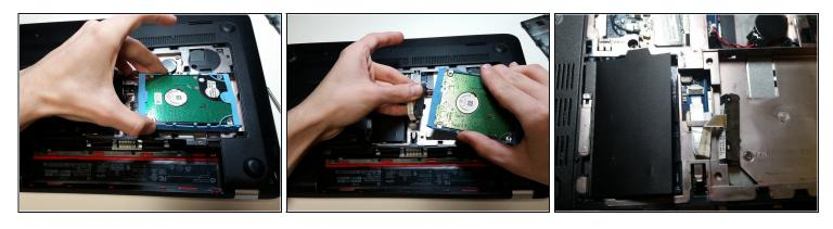
Remove the hard drive and disconnect its ribbon cable from both the hard drive and the motherboard.
