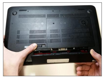
Slide the switch to release the battery and remove it.
