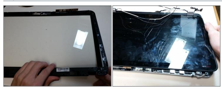
• Using a pry tool as necessary, remove the digitizer from the rest of the screen panel. Be careful around the top edge as there are delicate components beneath.
