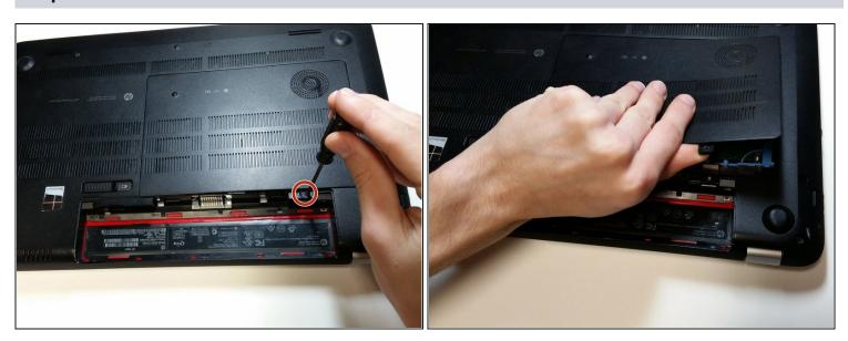
Remove the screw from the access panel. Gently lift and remove the panel.
