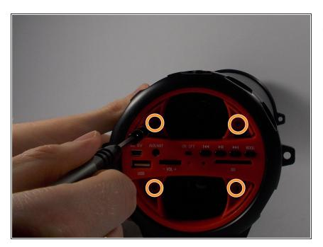
Remove the four 5 mm screws from the red panel under the mesh using a Phillips #1 screwdriver.
