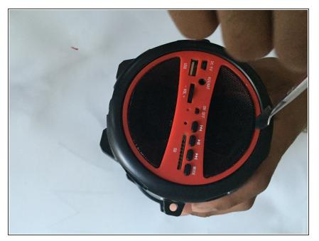
• Use a metal spudger to remove the mesh speaker covers (the side with the buttons) by wedging the narrow end into the center of the outer edge of the mesh, touching the red plate.
