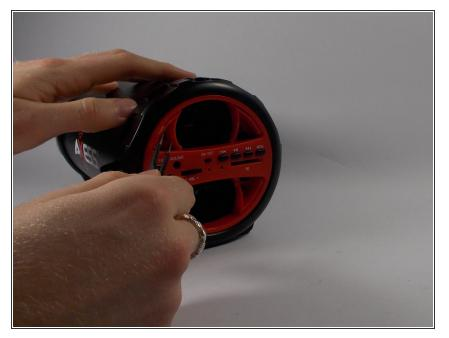
If the screws are difficult to remove, use a pair of tweezers to twist and pick them out.
