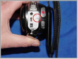
Remove all screws by walking around the unit. Be careful some are hidden under the handle, behind the hatches ....
