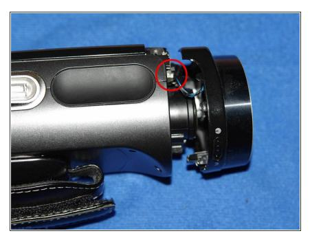
Then gently pull on the block, be careful it is connected to the camera by rather short cables.
