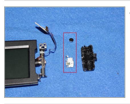
When reassembling, first position the metal clip and the small magnet in the black housing, before putting it back on the metal shaft.
