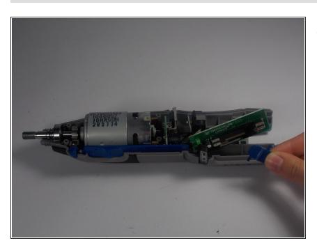
The speed selector switch is now easily accessible. Grab the switch and lift it out of the circuit board.
