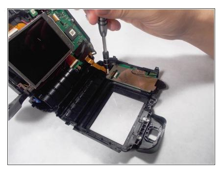
Open up the camera by removing the four 6 mm screws, that hold down the metal cover, using the
