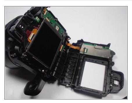
Proceed to insert and tighten screws around the screen which has been placed inside its metallic compartment. Be sure to screw in the main 0.4cm screw that connects both the LCD screen and metallic screen together first.
