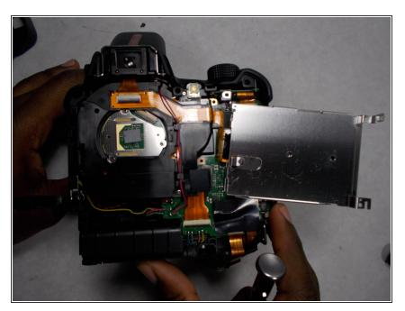
Disconnect the faulty screen from the metallic compartment as well as the motherboard of the camera.
