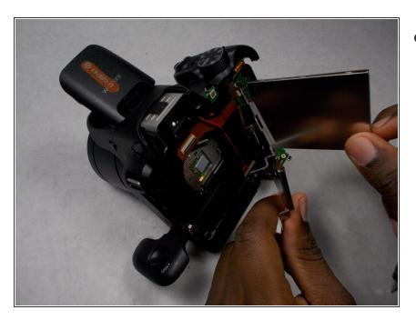
The LCD screen has two layers; the screen on top and the metallic screen protector it lays in. Make sure to take out the screw to the right of both layers that link them together.
