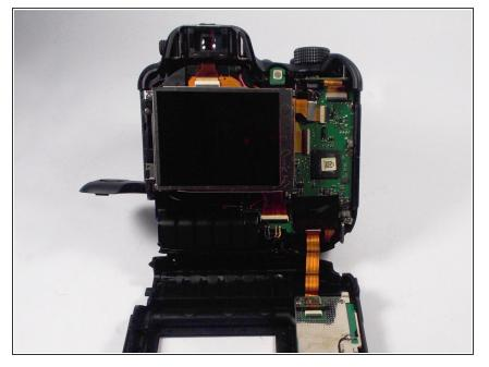
Place the new screen inside the metallic compartment and make sure it fits perfectly on each side.
