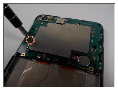
Using the PH000 screwdriver head, unscrew the screw that is holding down the motherboard. It is located on the left side of the motherboard.
