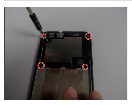
Using the T5 screw driver, unscrew all of the screws that are holding down the black plastic casing.
