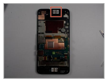
Once you have flipped the motherboard over, you should be able to locate the speaker at the top of the phone.
