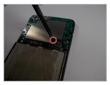
Using a pair of tweezers disconnect the battery from the motherboard so that the motherboard could later be removed from the device.
