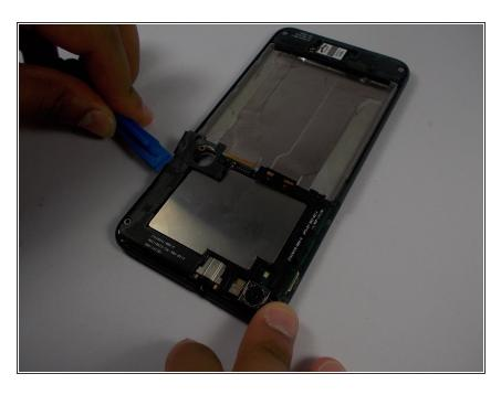
Remove the black plastics casing surrounding the motherboard with a plastic opening tool.
