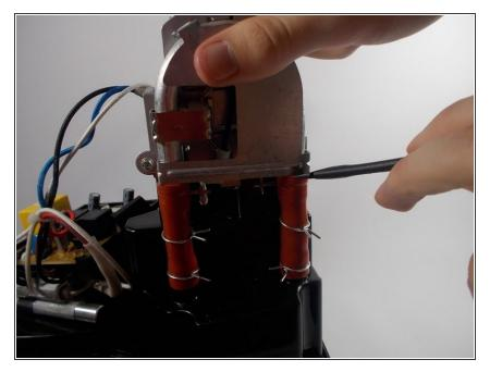
• After pushing the clips down, pull the tube from the heating unit. This may be difficult, so use a spudger to pry the tube off as you pull the unit up.
