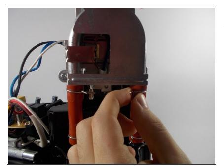
• Locate the top two spring clamps on the tube attached to the small heating unit. Pinch these clips while pulling down to release the tube from the heating unit. Pliers will make this task easier.
