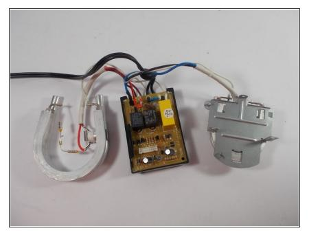
After removing the heating unit from the tube, the heating unit should come free. It will still be attached to the motherboard by three wires. They will be black, blue, and white.
