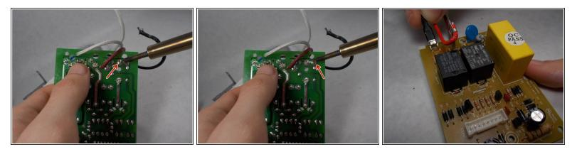
• First, remove the blue wire from the motherboard. This wire will have a black connector on the end connecting to the motherboard. It is found here. Heat up the solder on the bottom of the circuit board and remove the wire from its connection.
