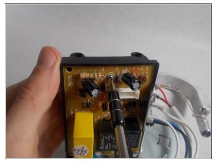
In order to remove the small housing that covers the motherboard, remove the lone screw with a PH1 bit. After this the plastic cover should easily snap off.
