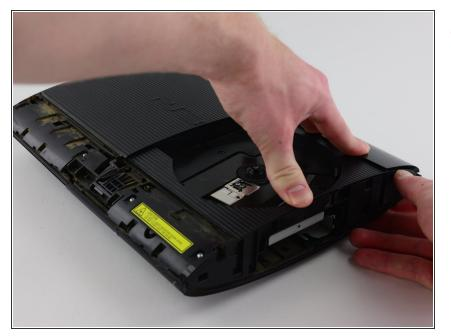
Remove the back panel by pressing down the tab on the right side of the device, and sliding the panel to the left.
