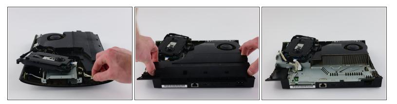
• Remove the cable from the plug and remove the wires from the two plastic hooks.
