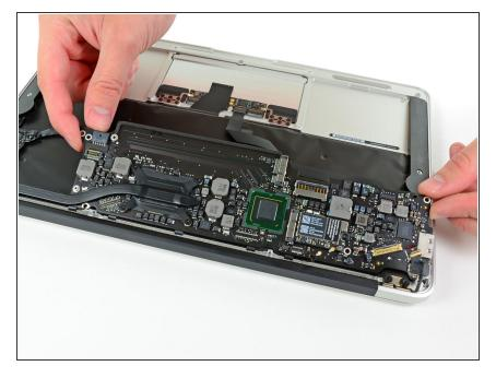
Gently lift the logic board assembly out of the upper case, minding the fragile heat sink and any cables that may get caught.
