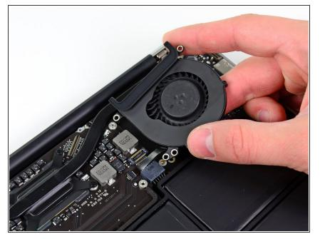
• Lift the fan out of the upper case and carefully pull the fan ribbon cable out of its socket as you remove it from the Air.
