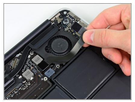
• Peel the I/O board cable up from the adhesive securing it to the fan.
