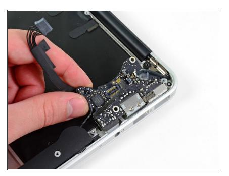
• Carefully lift the I/O board from its edge nearest the logic board and remove it from the upper case.
