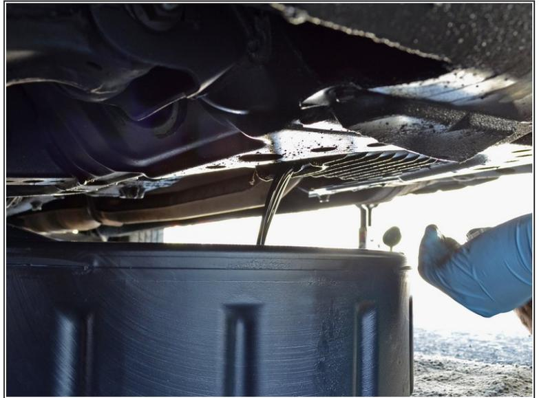
**!** Always wear protective gloves and eyewear when working with motor oil. Be careful if your car has been running recently as the engine and transmission may be very hot. Keep rags or towels nearby to wipe up any spills.
