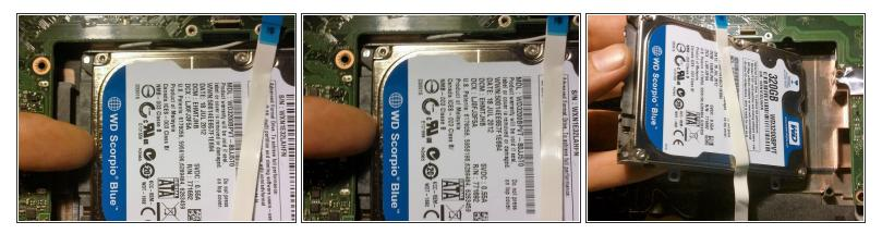
• Using a finger you can now slide the hard drive out
