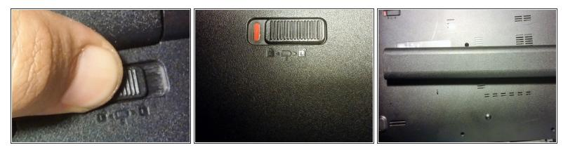
• Slide battery lock to unlocked position on left side, then hold it in on the right side while sliding the battery out.
