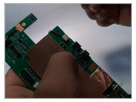
• Remove the USB port from the circuit board.
