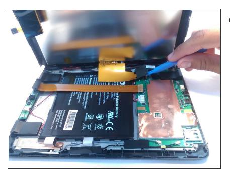
• Use the plastic opening tool to disconnect the LCD screen.
