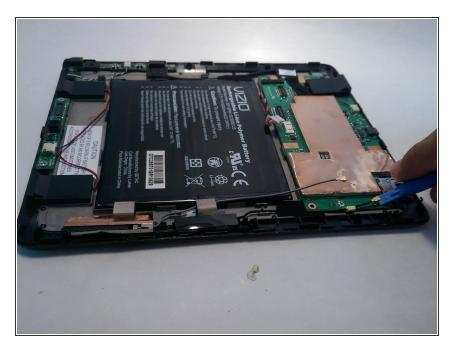
Use the plastic opening tool to disconnect both of the volume buttons.
