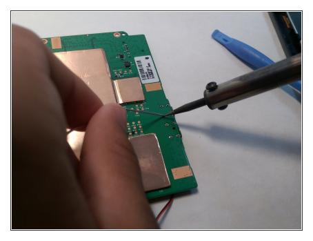
• Lastly, fuse the USB port back onto the circuit board.
