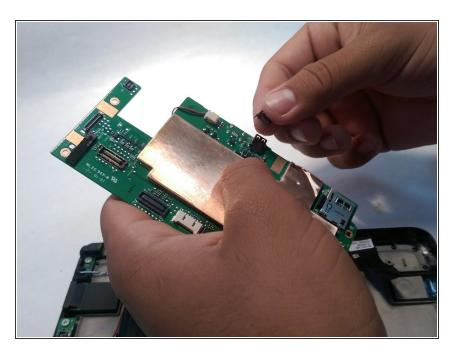
Insert the new USB port onto the circuit board.
