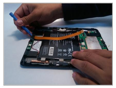
• Use the plastic opening tool to disconnect the camera.
