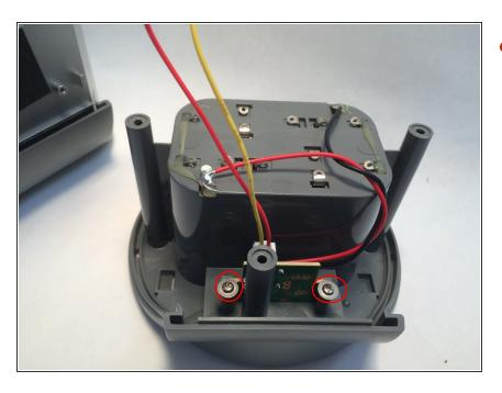
Remove both of the screws holding the power socket to the bottom chassis.
