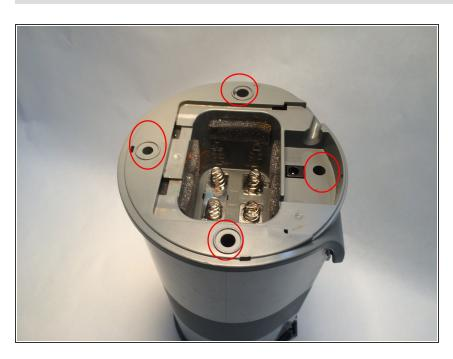
Locate and remove the four screws under each of the pads near the power socket.
