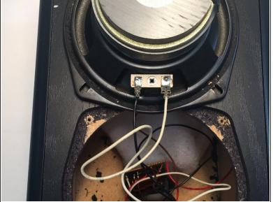
Once the speaker is removed, remove the black and white wires.
