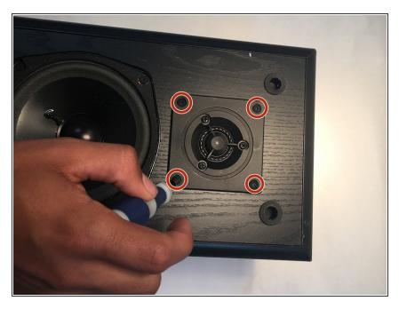
Once the mesh is removed, begin to remove the screws securing the small upper speaker/tweeter with a #1 Phillips head screwdriver.
