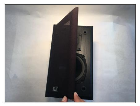
Remove the front speaker mesh to expose the speakers. The mesh will lift off without the use of tools.
