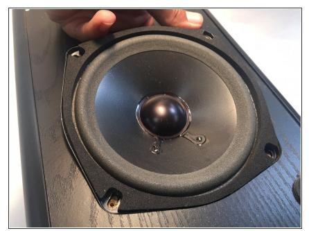
Once the screws are removed, remove the speaker by either prying up from the top, or pushing the speaker through by pushing on the bottom of the speaker.
