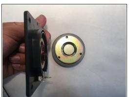
Remove the speaker from its plastic bezel using a #1 Phillips head screwdriver.
