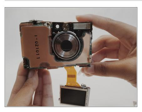
Remove the screws on the copper facing from the front part of the camera. Beneath is a connection to the screen. Wiggle this connection to pull it out; it may take some force to do so.
