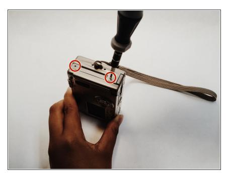
Using a Phillips #0 head screwdriver, remove the screws on the outside casing of the camera.
