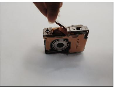
Remove the metal shield and screws from the bottom interior of the camera.
