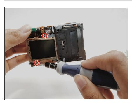
Use the Phillips head screwdriver to remove the screws securing the screen.
