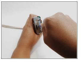
Use a pry tool to open the outer casing of the camera and access the internal components.
