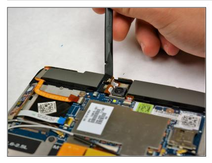
Use the Spudger to disconnect the ribbon cable to the upper camera by prying the connector away from the board.
