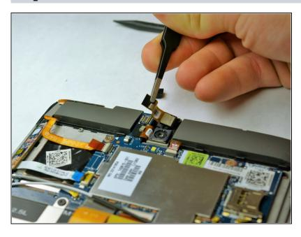
• Use ESD safe <u>tweezers</u> to pry the camera away from the motherboard starting at the side opposite the ribbon cable.
