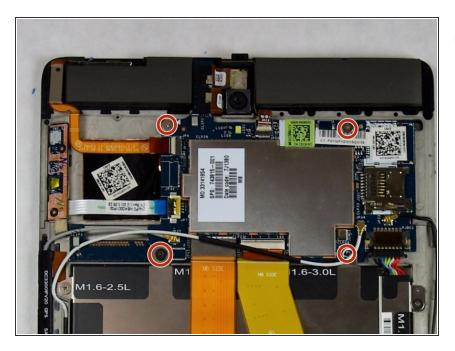
Remove the four PH#00 2.4mm screws that hold in the motherboard in place.
