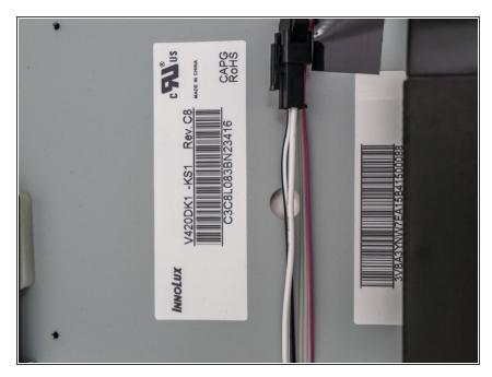
Model number of Innolux 3840\*2160 panel. It can support 60p/60Hz if you replace the driver board with one from Alibaba I think, according to its datasheet.
