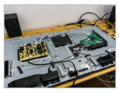
Removing some screws (Phillips) off the back panel allows it to be removed.
