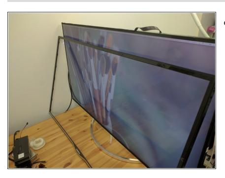
The display can be debezeled by removing all screws from back, and then sliding the brackets to the side gently to release. Top side needs some prying to release. Border is 9mm after mod.
