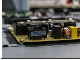
● This is the power supply. The output voltages include 24V (Backlight), 12V (Control + Panel).
