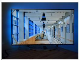
• Final result. Uneven lighting due to display is at an angle with the wall.
