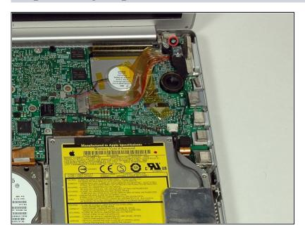
Remove the 12 mm Phillips screw holding the right speaker assembly to the lower case.
