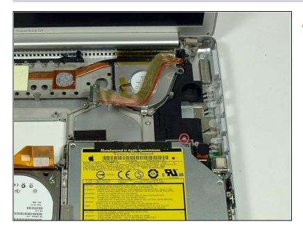
• Remove the single silver Phillips screw holding the right speaker housing to the lower case.
