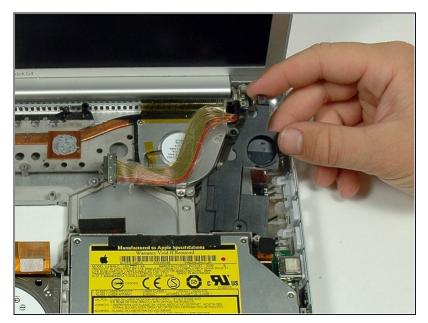
• Remove the speaker housing from the lower case.
