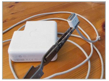
Start by examining the cable for any obvious cracks, holes or exposed wires
