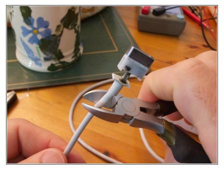
Having determined the likely source of the problem we need to remove the plug from the wire to see if the charger still works
