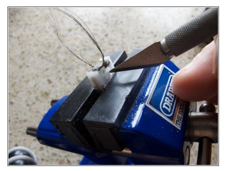
The first step is to carefully cut away the plastic moulding which is probably used as a diffuser for the status LED
