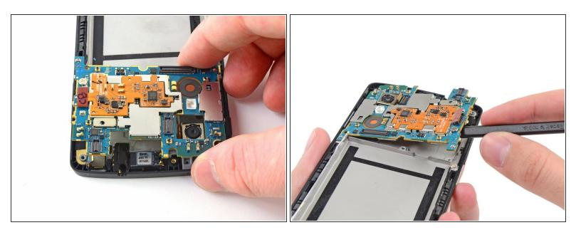
Gently lift the motherboard up and out of the device.
