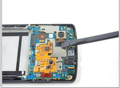
• Use the flat end of a spudger to disconnect the ribbon cable that connects rear-facing camera to the motherboard.
