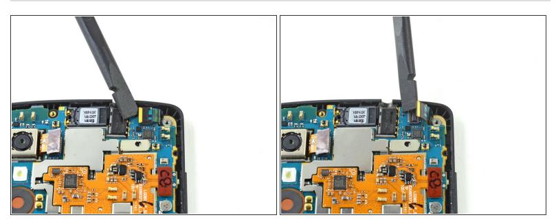
Use the flat end of a spudger to disconnect the front camera ribbon cable.
