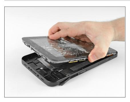
Lift and remove the front panel assembly from the rear panel.
