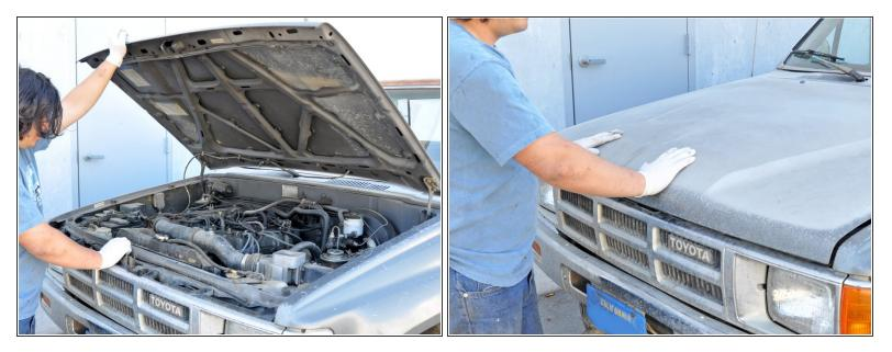
• Support the hood with one hand and use your other hand to place the hood prop rod back into its holder.
