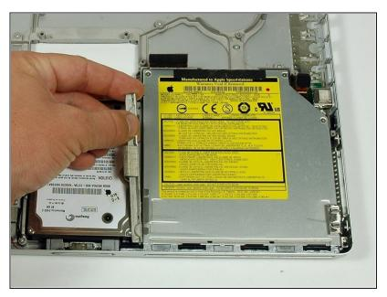
• Remove the retaining bracket.
