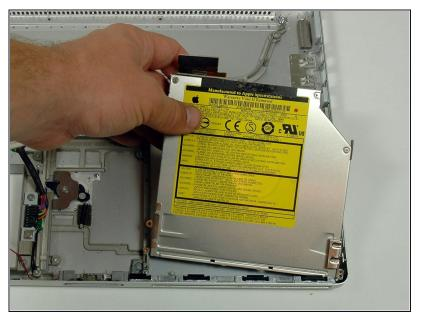
• Lift the optical drive out of the computer from the side with the connector on it.
