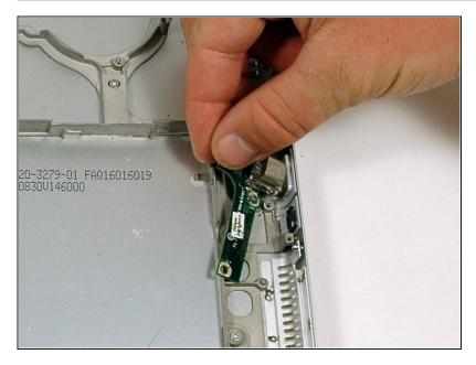
• Lift the USB board out of the lower case.
