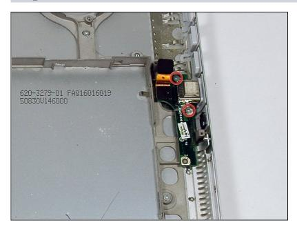
Remove the two 4 mm Phillips screws holding the USB board to the lower case.
