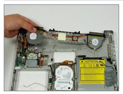
• Lift the heat sink and fans out of the lower case.
