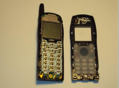
To separate front of phone from the back; start prying from bottom and work up the side. The phone should then pop apart.
