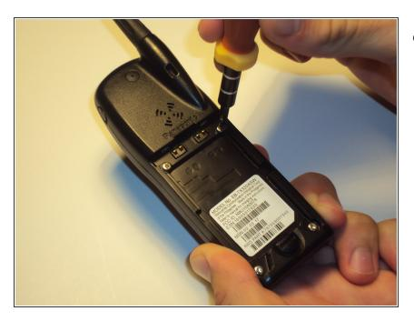
Using a Star 3.0 bit, remove 4 screws in battery compartment.
