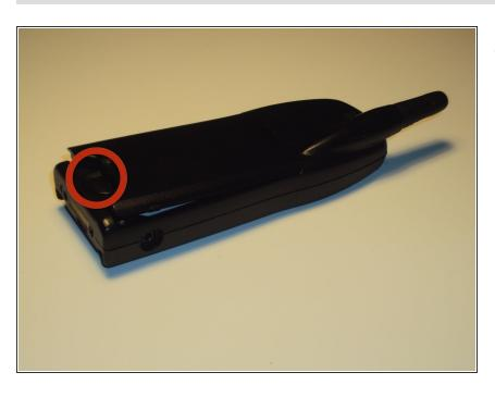
To remove battery push clip in; battery will pop out.
