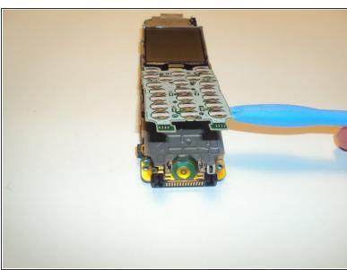
To remove keyboard circuit press on the middle and slide down. The board will pop up allowing for removal.
