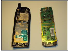
• To remove main-board from phone grab side of phone and pry upwards. Board should snap out.
