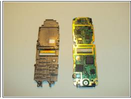
To remove main-board from bracket, gently apply pressure to the four small clips. Board will pop out freely.
