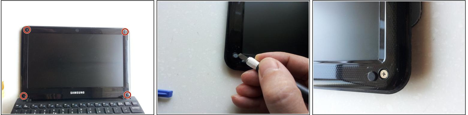
**⚠** For some reason the knife is the only way to get the correct angle and pressure to make the rubber feet release. Use of other tools is not recommended.
