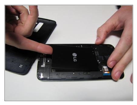
Push against the battery on the bottom, to take off the battery.
