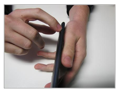
Push the bottom case in firmly with both hands to secure the case back onto the phone.
