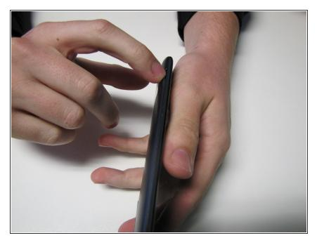
Insert thumb or any other thin flat object into the slight indent on the right of the phone.
