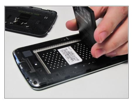
Align the new battery with the 4 bronze metals on the top left side of the battery and insert the new battery.
