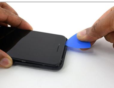
Slide an opening pick along the top edge of the iPhone, between the rear case and front panel, to break up the remaining adhesive holding the screen in place.
