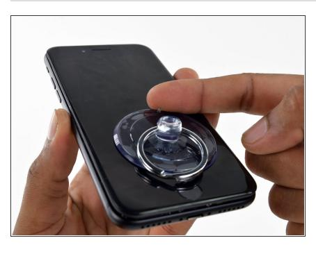
Pull up on the small nub on the suction cup to remove it from the front panel.
