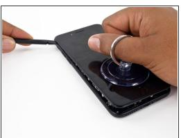
Slide the spudger up the left side of the iPhone, starting at the lower edge and moving towards the volume control buttons and silent switch.
