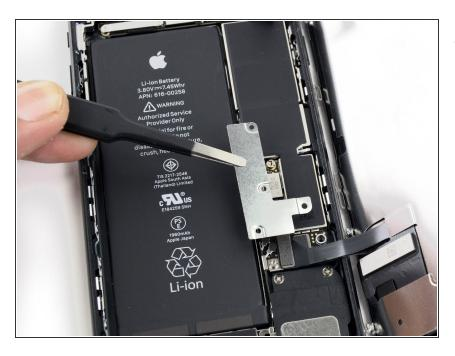
Remove the lower connector bracket.
